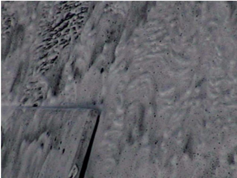
**Figure 6:** Close up of foam adhesion to vertical surface fire-fighting foam on aircraft surfaces.
