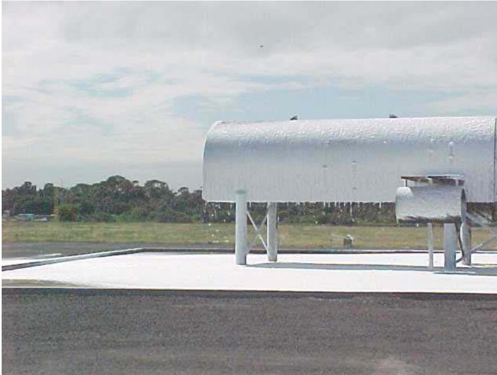
**Figure 5:** Foam adhesion to vertical surface.
