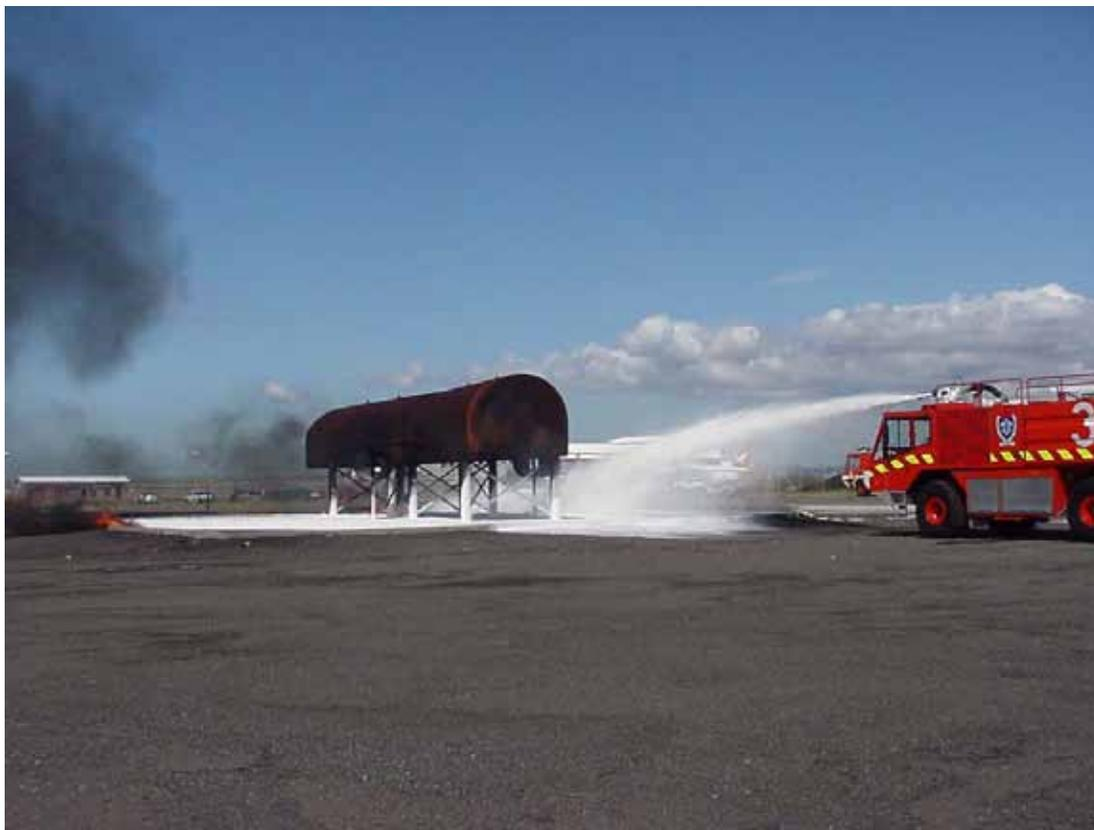
**Figure 1:** 3M RF6 foam being tested through ARFF vehicle.
